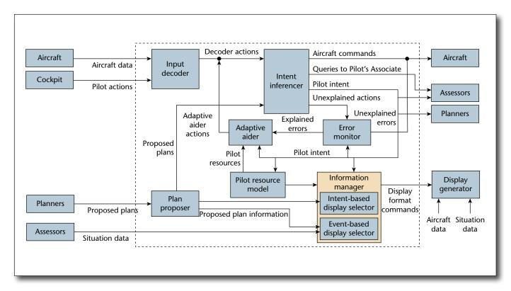
Figure 6. Flowchart of the Demo 3 Pilot-Vehicle Interface.
