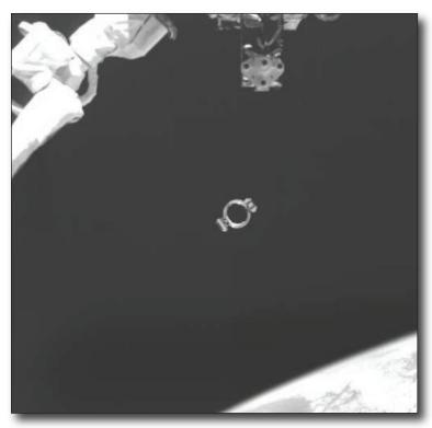
*Figure 2. The Ejected Separation Ring.* NextSat (top) is at the end of the robotic arm (upper left).
