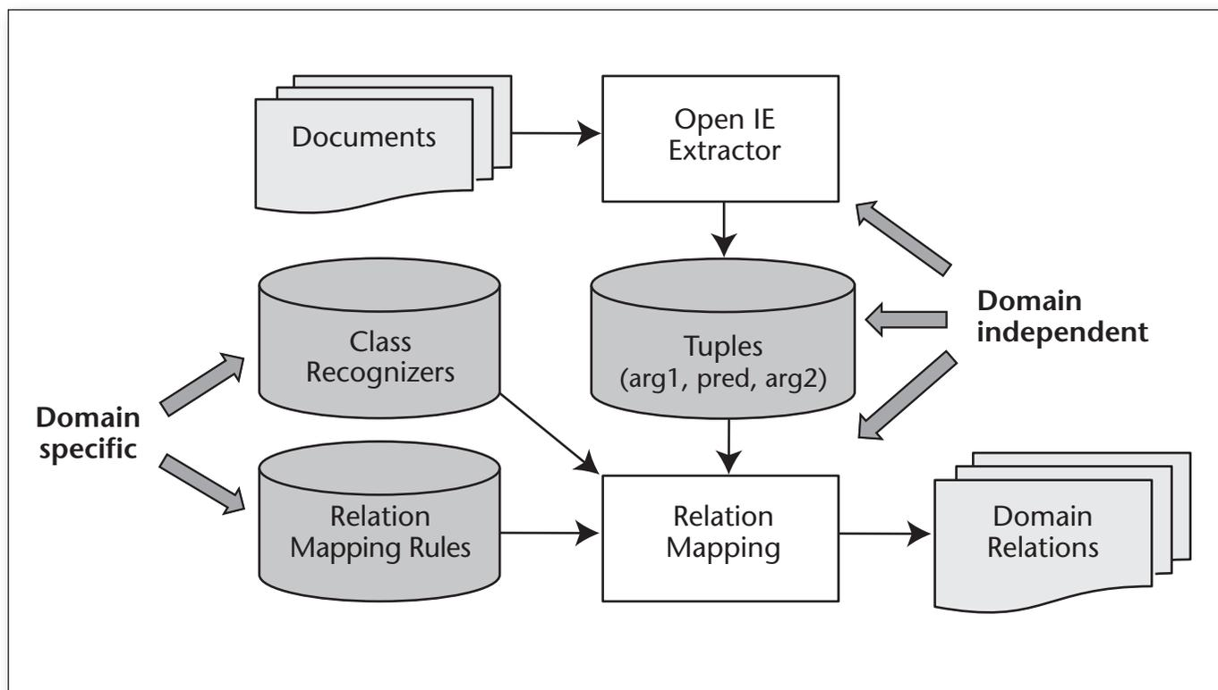
Figure 2. System Architecture.
