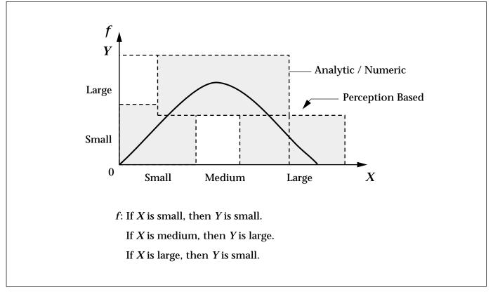
*Figure 5. Perception-Based Function Representation as a Collection of Linguistic If-Then Rules.* The granules in the (*X*, *Y*) space are Cartesian products of the granules in the *X* space and *Y* space.
