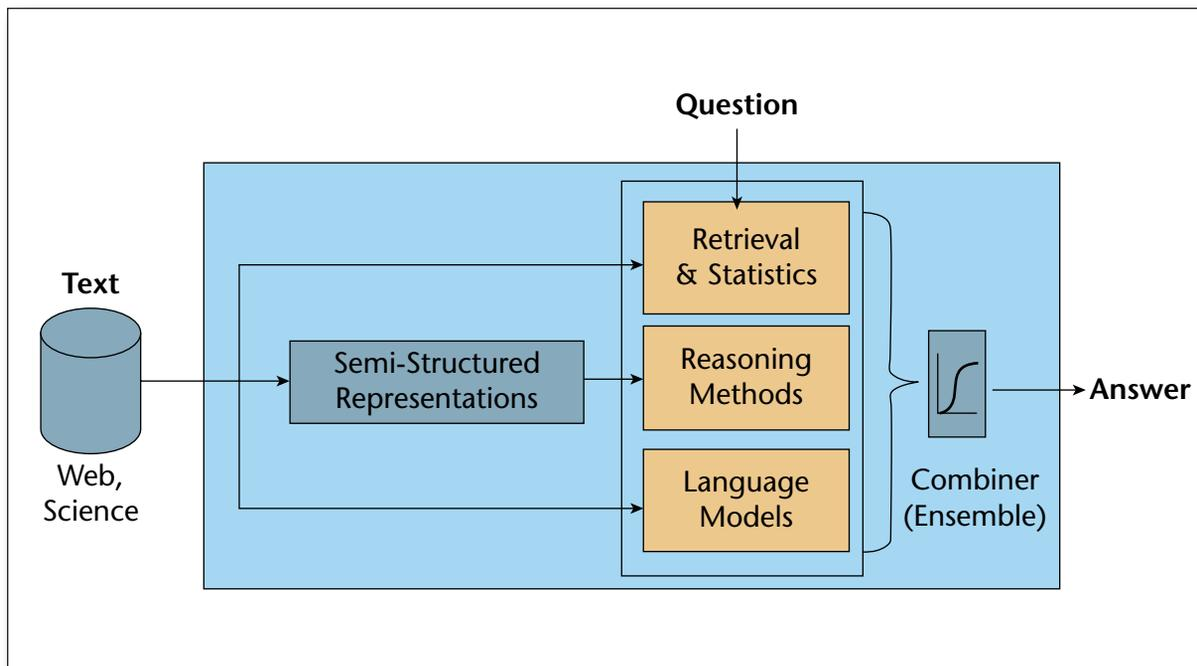
Figure 2. A Simplified Picture of Aristo's Architecture.
