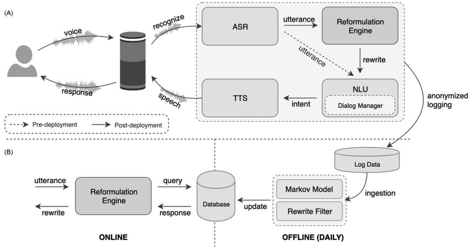
**FIGURE 1** A high-level overview of the deployed architecture with our reformulation engine in context of the overall system in (A) and the offline sub-system that updates its online counterpart on a daily cadence
