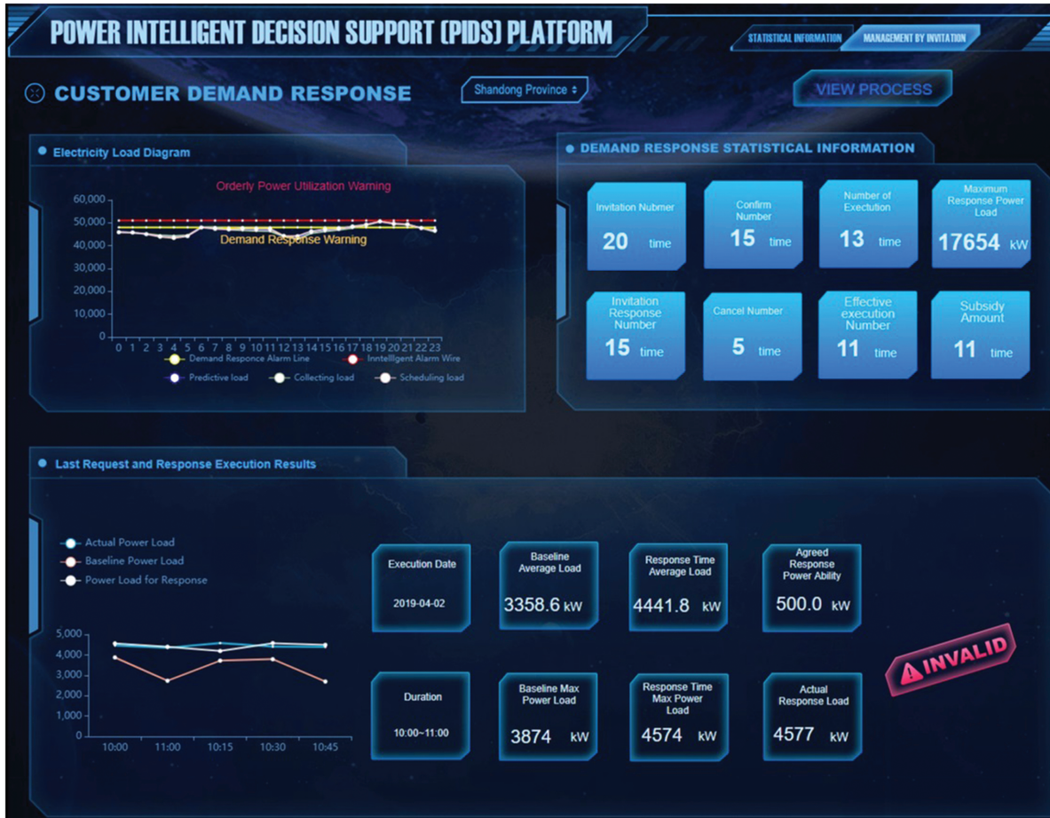
FIGURE 3 The PIDS user interface showing decision support functions related to demand response optimization (02-Apr-2019)
