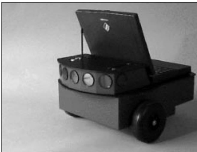
*Figure 1. A Pioneer Robot with Laptop Host Computer.*
