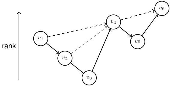
(a) Example CH  $G'$  with dashed shortcuts. The path  $\pi' = v_1 v_4 v_6$  in  $G'$  consisting of two shortcuts (dashed black arrows). The corresponding mimicked path in the original graph  $G$  (without shortcuts) is  $\pi = v_1 v_2 v_3 v_4 v_5 v_6$ .
