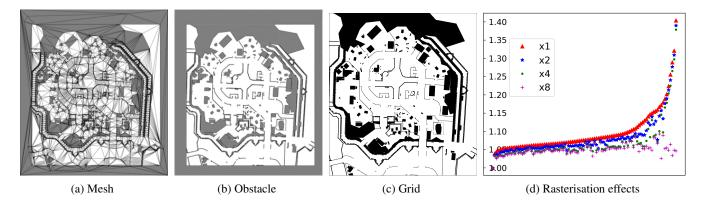
Figure 2: We show examples (2a-2c) of different map representations for the level scene\_sp\_sax\_07. We also report (2d) the effect that grid resolution has on path length (grid-optimal vs mesh-optimal) for a set of 100 co-solvable instances.
