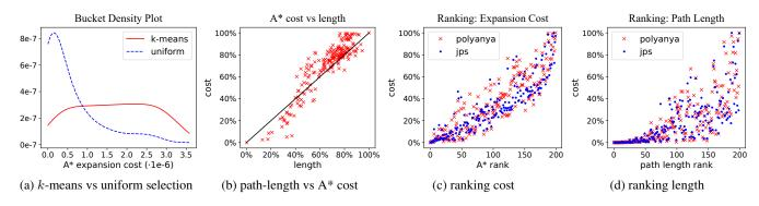
Figure 3: Clustering efficacy for the map scene\_sp\_sax\_07. We look at the distribution of selected instances in Figure 3a and the rank of each instance according to A\* expansion cost and path length metrics, in Figure 3b. In Figures 3c and 3d, we analyse how well the A\* expansion cost and path length ranking compare to the expansion cost rank of different planning algorithms (here, for improved clarity, we only plot every 10th instance).
