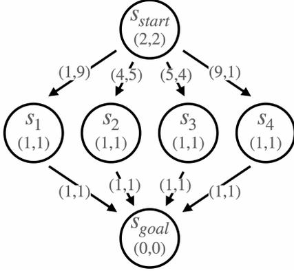
Figure 3: An example problem instance whose Pareto-optimal frontier consists of four paths. The pair of numbers inside each state is its  $h$ -value. The pair of numbers annotating each edge is its cost.
