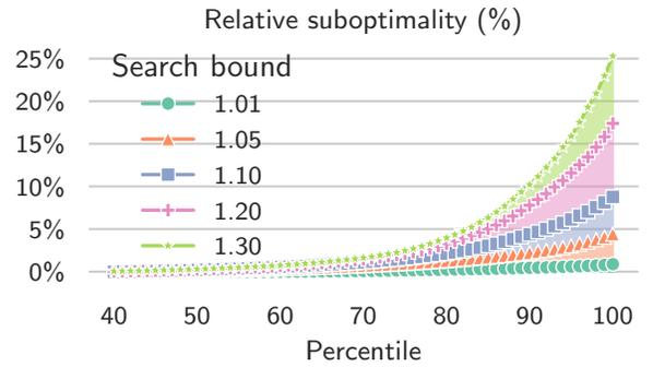
Figure 7: Percentage difference between the optimal path and suboptimal paths found for different admissibility percentage (% sub-optimal).
