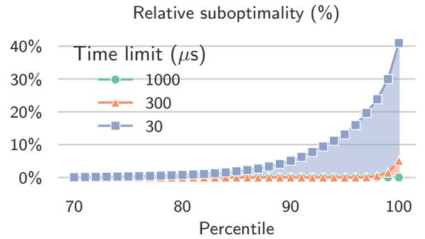
Figure 9: Percentage difference between the optimal path and suboptimal paths found for different time limits ( $\mu$ s).
