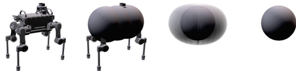
Figure 2: Obtaining the collision-checking geometry of a subspace XYZ which discards yaw rotations from the full space XYZ \theta . Left to right: the robot, the collision geometry in the original state-space, geometries of densely sampled states (varying yaw), intersection of all geometries. The collision-checking geometry used for this subspace is a sphere.
