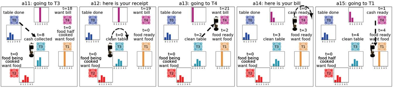
Figure 4: Example output policy for  $H = 4$  and 5 tables. The histograms show the belief over satisfaction for different tables. The leftmost bar is 0 (very unsatisfied) and the rightmost is 5 (very satisfied). The robot’s action is shown on top of each figure. Each table’s request and the amount of time they have been waiting is shown above it.
