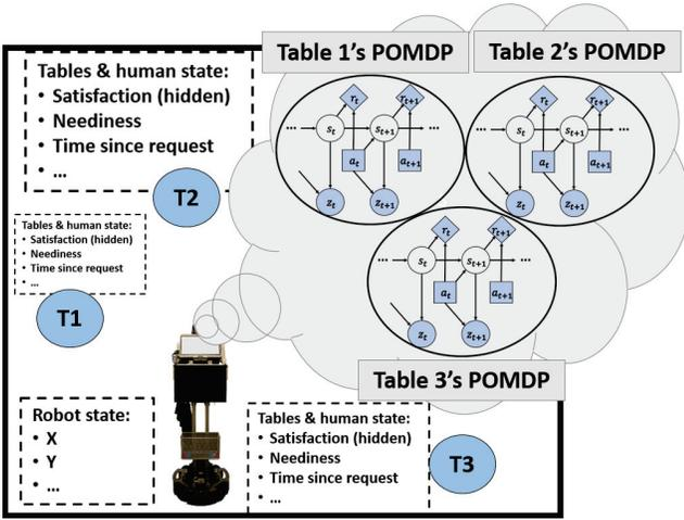
Figure 1: The robot operates in a restaurant with 3 tables,  $T1$ ,  $T2$ , and  $T3$ . The robot builds a POMDP model for each table in the restaurant by using its own state and service actions, the table's state and the human's state. The robot has  $N$  POMDP models for a restaurant with  $N$  tables.
