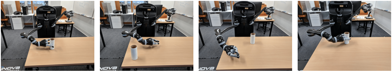
Figure 3: Snapshots of a successful run with two obstacle position changes. The robot attempts to pick-up the cup (first picture) but the cup position is changed to the left corner of the table (second picture). It performs a scan action, and attempts to pick up the cup again. But, the cup is again moved to a location close to the robot (third picture). A scan action is performed again. In the last picture the robot successfully picks-up the cup at its the new location.
