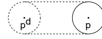
Figure 1: A stadium formed from a circular agent ( p ) and its delayed position ( p^d ).
