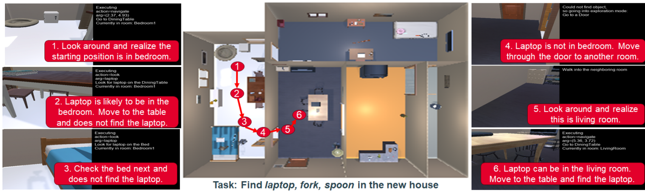
Figure 1: A SayNav example: The robot uses LLM-based planner to efficiently find one target object (laptop) in a new house.
