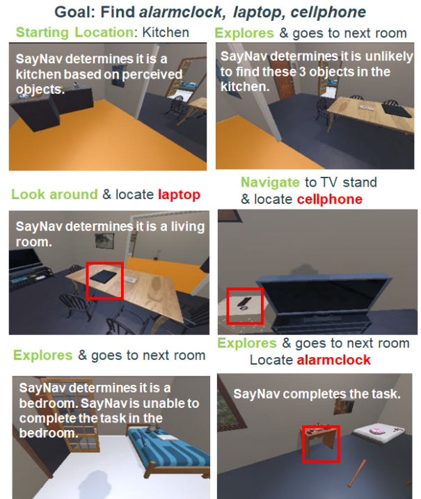
Figure 7: Visualization of an episode with SayNav (OrNav + GT) for multi-object navigation task.
