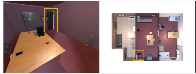
Figure 10: A failure example: The left picture shows the RGB image from the camera mounted on the agent and the right picture shows the top-down view of the house. Due to geometry of the room, agent is unable to observe that the door is open and hence, unable to navigate through the door (marked with yellow rectangle).
