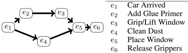
Figure 1: Partial Order for a windshield installation task in an automobile manufacturing facility. Events  $e_1, \dots, e_5$  represent events such as “car arrived” ( $e_1$ ) or the commencement of various tasks such as “clean dust” ( $e_4$ ).
