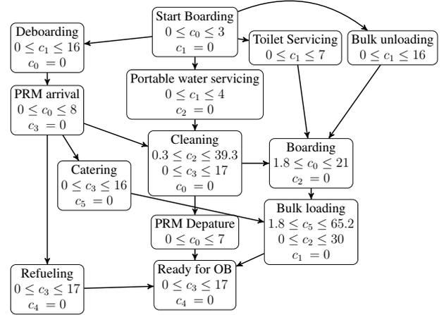
Figure 6: Mined TPO for aircraft turnaround.
