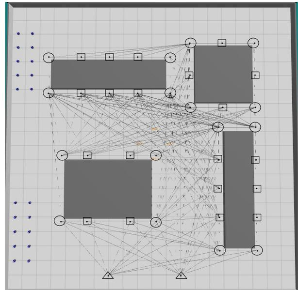
Figure 6: Factory map used in the experiments, containing four static obstacles, 20 workstations ( $\square$ ), 16 waypoints ( $\circ$ ), and two drop-off stations ( $\triangle$ ). 20 AMRs are placed in two groups to the left.
