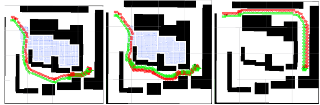
Figure 3: Results with h_b using w=100 (left), h_b using w=10000 (center) and h_{ed} (right). Left footsteps are marked as red, right footsteps are marked as green and states expanded during search are marked as blue.
