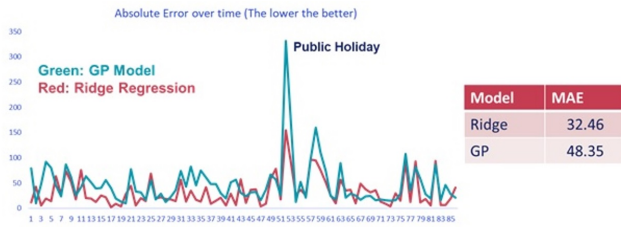
Figure 4: Comparing the error over 12 weeks of data, the noise introduced by region boundaries results in inferior performance predicting overall counts for the GP model.
