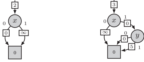
(a) A symbolic state represented as EVMDD \mathcal{E} with the corresponding cost a state is reachable with. (b) The resulting symbolic state represented by EVMDD \hat{\mathcal{E}} = \text{image}(\mathcal{E}, T_a) . T_a is shown in Fig. 3.
