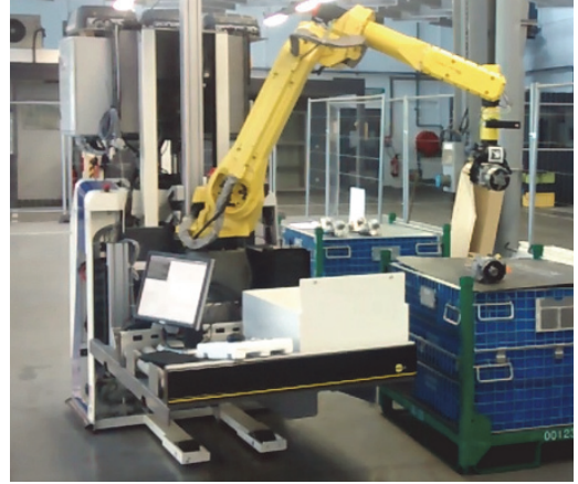
Figure 1: A robot operating in a factory environment using the integrated system. The robot is executing a six-step plan to place two parts in the white kitting box it is carrying.
