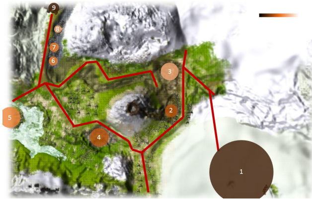
Figure 6: Specification of search paths and areas in a simulated environment (tablet interface). The red segments are possible paths followed by missed hikers, darker areas are associated with a higher priority value.
