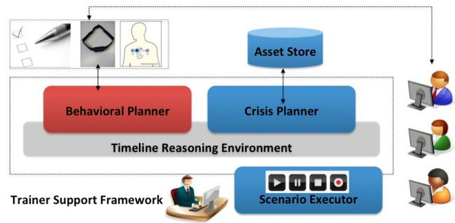
Figure 1: The PANDORA architecture. The Crisis Planner and the Behavioral Reasoner are the key components that share a common timeline-based reasoning structure.
