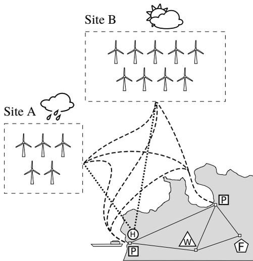
Figure 1: A typical wind-farm maintenance problem. Ships can sail along dashed routes, while helicopters can only leave from airports and move between wind-farms. Both ships and aircraft must *Enter* the site before being able to move amongst turbines, and *Exit* in order to return to port, making each wind-farm a restricted portion of the state-space. Nodes are labelled as follows: *H* – heliport, *P* – sea port, *W* – warehouse, *F* – factory.
