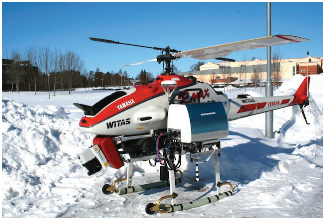
Figure 1: The Yamaha RMAX helicopter with integrated laser range finder mounted on a rotation mechanism.
