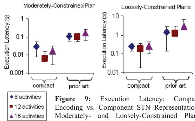
**Figure 9:** Execution Latency: Compact Encoding vs. Component STN Representation. Moderately- and Loosely-Constrained Plans encode 501-1500 and 1501-5000 feasible component STNs, respectively.
