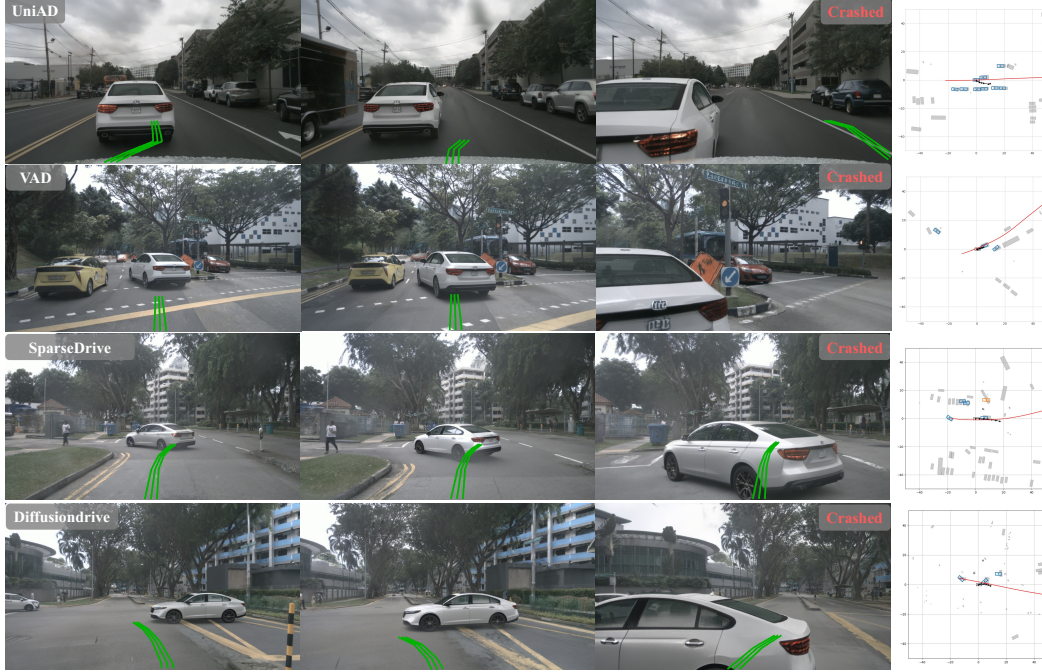
Figure 7: Qualitative comparisons of the failure cases of four E2E-AD models in handling corner cases within closed-loop simulation.
