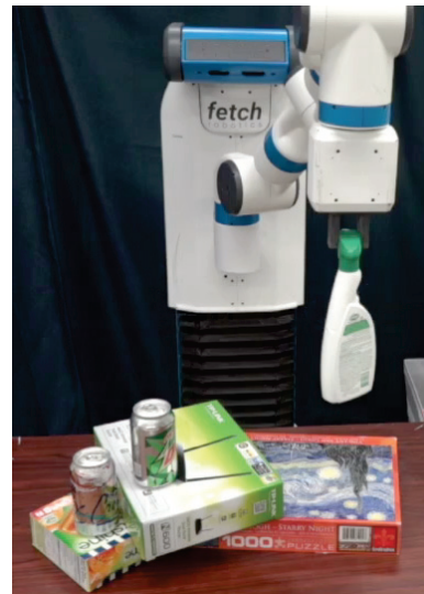
Figure 8: An example case study where the Fetch Robot successfully picked up a spray bottle based on an Amazon Mechanical Turk worker’s annotation using EURECA.
