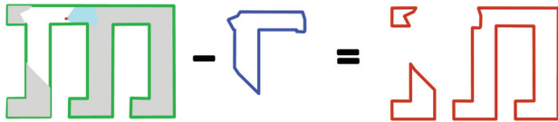
Figure 2: The covered region (blue) is subtracted from the overall space geometry (green) and result in the uncovered regions (red)
