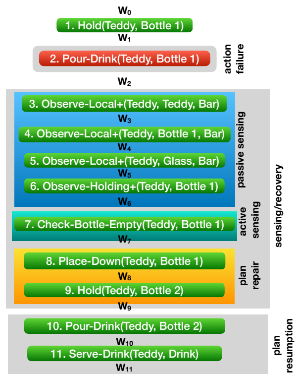
Figure 1: A solution plan for the Drink Refill domain's planning problem. Green actions are successfully performed actions. Red actions are ones that are attempted but that fail because their material preconditions are not all met in the world state where they are attempted.
