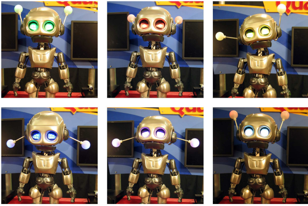
Figure 3: Quasi’s emotional expressions and corresponding eye/antennae colors; clockwise from top left: happy (green), angry (red), confused (yellow), neutral (white), embarrassed (pink), and sad (blue).
