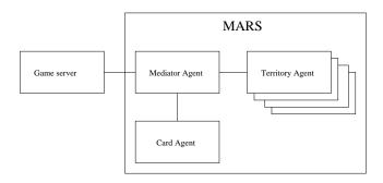
Figure 2: MARS Architecture.
