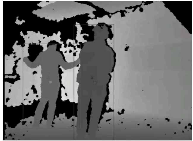
Figure 5: The depth map as seen by the Kinect camera in the interactive installation version of the Melody Triangle. The bounding box outlines the blobs detected by OpenNI.
