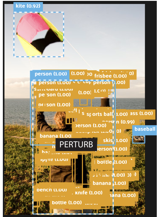
Figure 3: An untargeted attack perturbs a person and causes Faster R-CNN to miss the kite (and baseball) and hallucinate objects like bananas.
