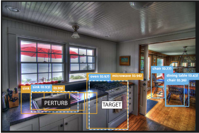
Figure 2: A mislabeling attack perturbs a sink and causes SSD to mislabel the targeted oven as a microwave with 0.96 confidence.
