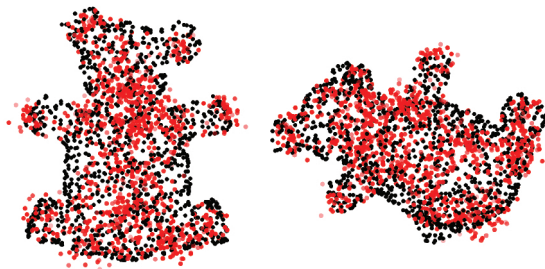
Figure 5: Black points are the subsampled input point cloud which is used to estimate the underlying generative model. Red points show sampled points from our underlying probabilistic model (the more opaque being more probable - best viewed using zoom).
