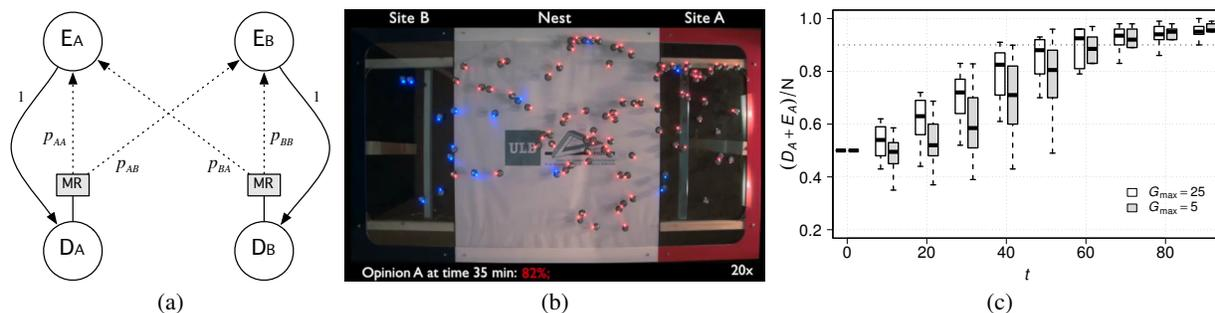
Figure 1: Illustrations of: a) the probabilistic finite-state machine of the individual agent; b) screen-shot of a robot experiment; and c) proportion of robots with opinion *A* over time during robot experiments.
