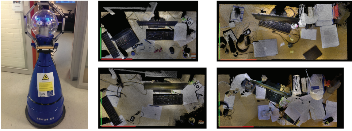
Figure 2: Column-1 (L to R) shows the robot ROSIE (SCITOS G5 platform with additional 3D sensors) that is being used for deploying and testing our current systems. Column-2 shows the table of the same person with changes in arrangement between the morning and evening on the same day. Column-3 shows the table configurations of a different person 12 days apart (Thippur et al. 2014).
