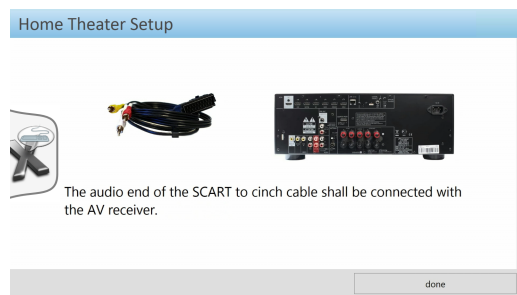
Figure 1: The figure shows a single user instruction that visualizes a single action of a solution plan. The respective ports of the audio/video receiver are flashing in red.
