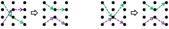
Figure 2: Two kinds of adjustment. Left: when two paths are crossing; Right: when two paths overlap.
