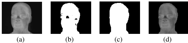
Figure 1: The first step in the proposed algorithm is to segment out the face. This removed image areas unrelated to the subject’s identity and aids in the convergence of the AAM. From (a) the original image (b) provisional segmentation mask is created using temperature thresholding, after which (c) morphological operators are used to increase the segmentation accuracy to outliers e.g. such as which occur at the interface of facial and non-facial regions, producing (d) the final result with the background correctly suppressed.
