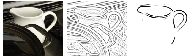
Figure 1: Example of shape matching under heavy occlusion. (left) Image window, (center) normalized gradient magnitudes, and (right) probability that each pixel matches the shape of the pitcher.
