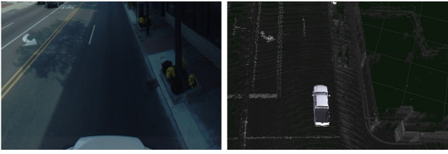
Figure 4: (left) Image with shadows of trees and buildings on the road. (right) Top view of the corresponding lidar reflectivity map, which is unaffected by ambient lighting.
