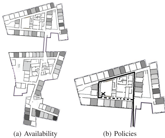
Figure 4: (a) Availability of humans in our building - darker gray represents higher availability. (b) The HOP-POMDP takes a longer route with more available people.
