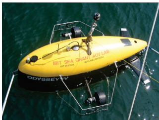
Figure 9: Odyssey IV, an AUV from the MIT AUV Lab at Sea Grant, is 0.7 \times 1.4 \times 2.2 m, weighs 500kg dry and about 1000kg wet, and has rated depth 6000m.
