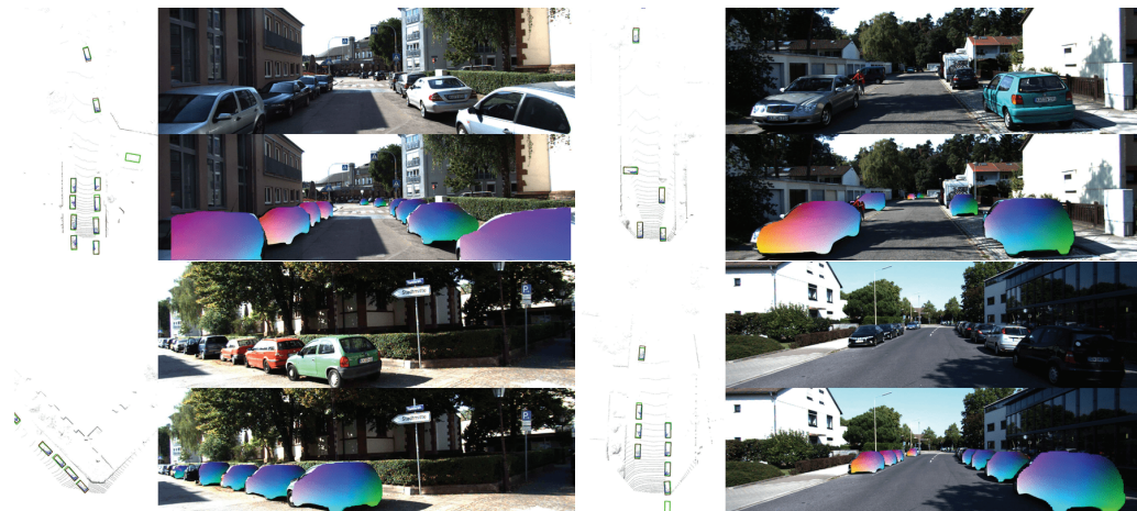
Figure 6: Quantitative results. For each example, the image on the left is the BEV map, the two stacked images on the right are the original left image and the visualization of predicted part locations on predicted masks. On the BEV image, the red box represents the detection box and the green one indicates the GT box. In addition, the GT LiDAR points are shown in gray while points generated by ZoomNet are shown in blue.
