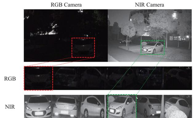
Figure 1: Examples of images captured by RGB and NIR cameras from six camera views. Middle: the RGB images of six camera views. Bottom: the corresponding NIR images.
