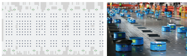
(a) The 2D grid layout of an automated sortation center. Green cells represent sorting stations. Gray cells represent obstacles. Blue cells represent sorting bins. (b) Robots delivering parcels to sorting bins (Reuters 2018).
