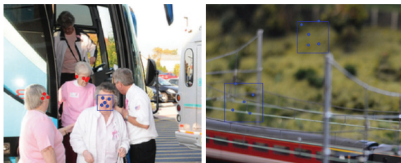
Figure 3: Example face and landmark detections from COCO validation set. (Left) Face detected (blue rectangle) and landmarks detected within the face (blue dots). The red dots represent undetected groundtruth face landmarks by the pipeline. (Right) False face detections and wrong landmarks within the rectangles.
